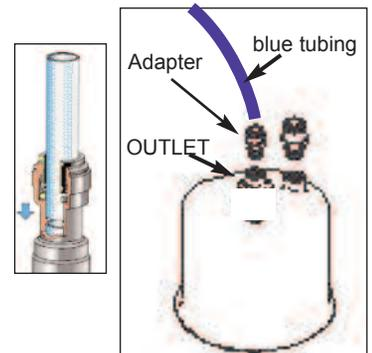
Insert tubing and push until you feel resistance -- at this point, the tubing is **not** fully inserted. Push firmly until the tubing is inserted as far as it will go.
