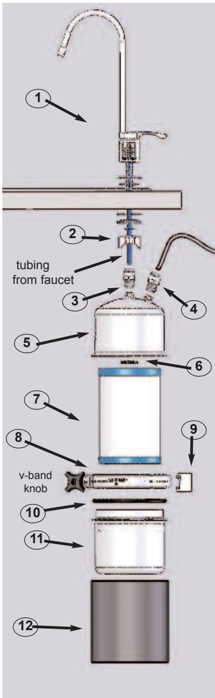
**Note:** the Aquaversa MP750SI Inline unit does not include the following parts: faucet assembly (#1), wing nut (#2), outlet adapter (#3), inlet adapter (#4), acrylic sleeve (#12), clear tubing (#13), adapta valve (#14)
